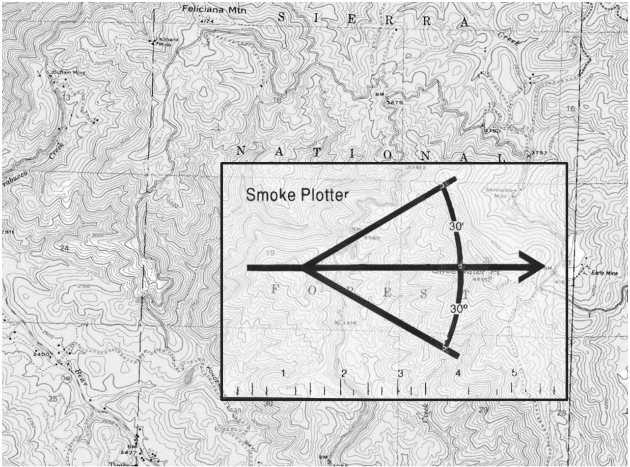
Figure D1 Smoke Plotter (NWCG RX 410)
